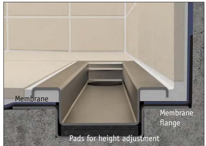
Tiles and liquid membrane
